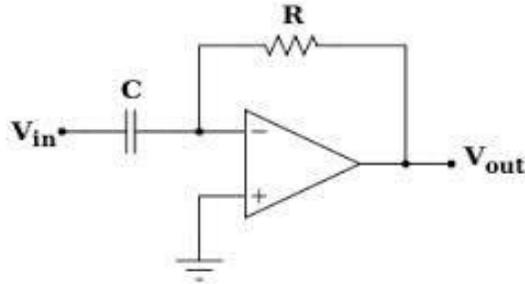
$$V_{out} = -RC \left( \frac{dV_{in}}{dt} \right)$$
