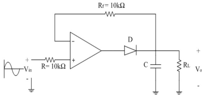
20. **Determine the output voltage for the circuit shown in fig when a)  $V_{in} = -2V$  (b)  $V_{in} = 3V$ . (ID)(Nov 2015)**
