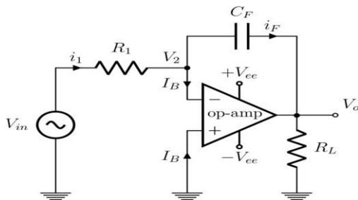
$$v_o = -\frac{1}{R_1 C_F} \int_0^t v_{in} dt$$
