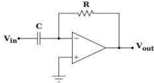
$$V_{out} = -RC \left( \frac{dV_{in}}{dt} \right)$$
