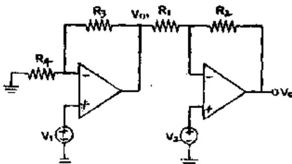
11. Draw the circuit diagram of an instrumentation amplifier and explain its operation .list few application? D (12)(A/M 2016)
