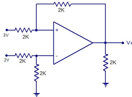
24. **Calculate the output voltage for the circuit shown below. (ID)(May2016)**
