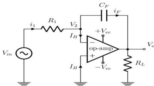
$$v_o = -\frac{1}{R_1 C_F} \int_0^t v_{in} dt$$
